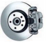
The system comes with four disc brakes with active sensors, brake servo with additional chamber and floating callipers, double crossover circuit. ABS with four channels and four sensors and EBD (Electronic Brakeforce Distribution) allowing maximum control of the vehicle during the braking action.
