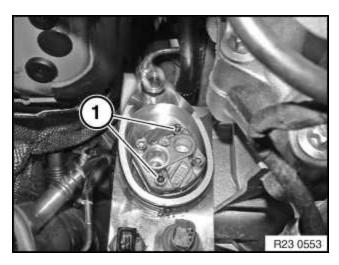
17. Release two M5x40 Allen head screws (1) of the hydraulic pump, as shown on the illustration. Gently (using small screwdriver) pry-out the pump out of the housing.
