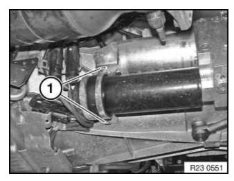
18. Release two Torx M8x25 bolts (1) of the accumulator bracket.
