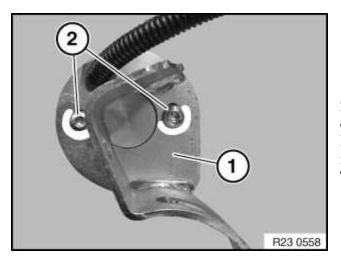
23. Install bracket holder (1) at the back of the new electric motor using two M5x12 Torx screws (2) provided in the motor repair kit (P/N 23 01 7 841 032). Torque to 5 Nm.
