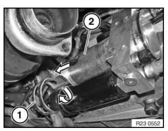
20. Release (bend) accumulator retaining clip (1) and move electric motor (2) forward, to separate it from the hydraulic unit housing.
