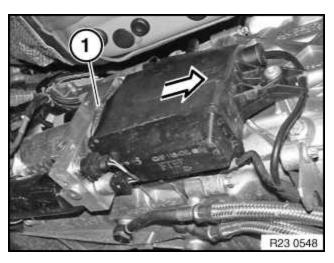
15. Release clamp (1) between hydraulic unit and fluid reservoir.
