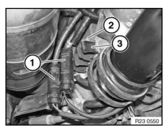
12. Unclip oxygen sensor connectors (1), release nut (2) and remove bracket holder (3) to gain an access hydraulic accumulator bracket.
