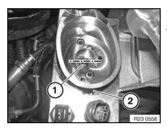
25. Use new M5x20 Allen screws provided in the motor repair kit (P/N 23 01 7 841 032). Torque to 6 Nm.
