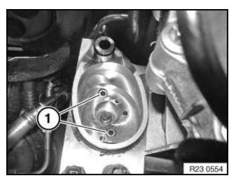
19. Remove two M5x20 Allen head bolt (1) holding motor to hydraulic unit housing.
