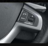
Bluetooth<sup>®</sup> for compatible mobile phones Integrated Bluetooth<sup>®</sup> allows you to receive calls with compatible mobile phones – hands-free – via the steering wheel controls. The audio system even mutes automatically when a call comes in.
