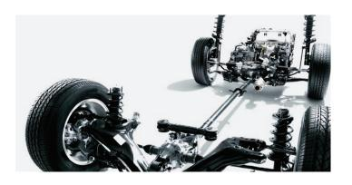
The Intelligent Control System instantly assesses the slope of the road angle using a sensor and uses the VSA system to assess the available grip, providing additional rear torque where necessary to ensure a smooth take off.
