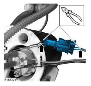
${\bf 8.}$  Using a suitable tool, remove 5mm of insulation from the end of each wire.
