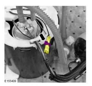
13. CAUTION: Make sure the wiring is cut as close to the connector as possible.
