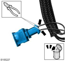
14. Using a suitable tool, remove 5mm of insulation from the end of each wire.
