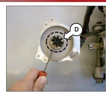
5. Install the new improved flexible coupling onto the steering column.
