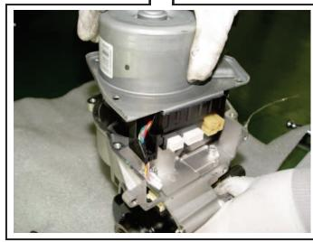
12. Remove the original flexible coupling (O) from the housing. In addition, use an air gun to remove any foreign matter from the motor and/or the housing.
