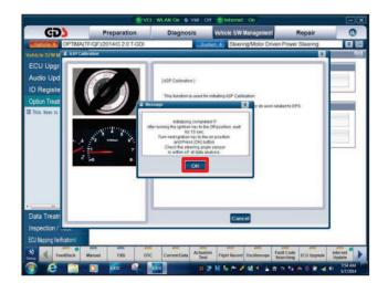
11. Access **Current Data** and verify the Steering Angle Sensor value is at 0.0 ± 5.0 degrees.
