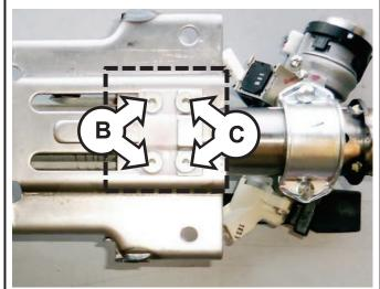
Lift the steering column guide bracket
