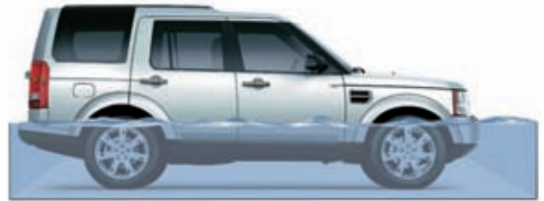
Wading Depth (in off-road mode) Maximum wading depth 700mm (air suspension only) Normal wading depth 600mm
