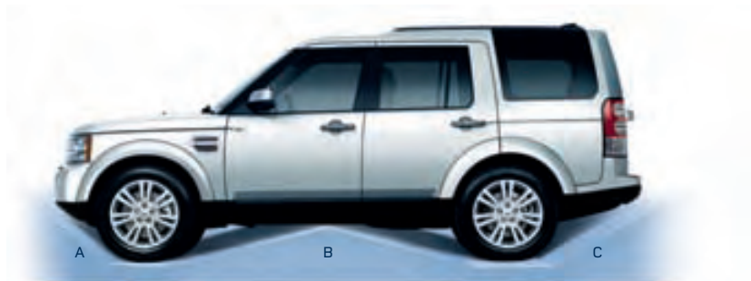
Off-road Geometry A B C Approach Angle 36.2° 27.3° 29.6° Ramp Break Over Angle Departure Angle Off-road ride height (air suspension)
