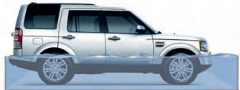
Wading Depth Maximum wading depth 700mm (air suspension only) Normal wading depth 600mm
