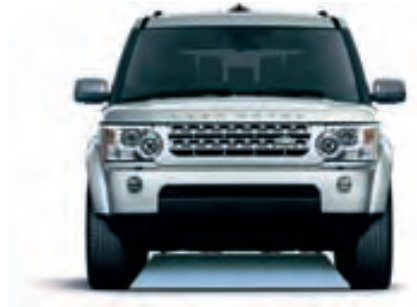
Obstacle Clearance Ground clearance up to 310mm (air suspension) Standard ride height 185mm
