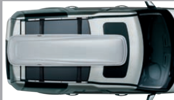
Sports Box* VPLDR0002 Lockable for security. Can be mounted either side for kerbside opening in any country. Internal retention system for skis or other long loads. External dimensions: 2,300mm long, 620mm wide, 390mm high. Volume 400 litres. Load capacity 56.3kg.
