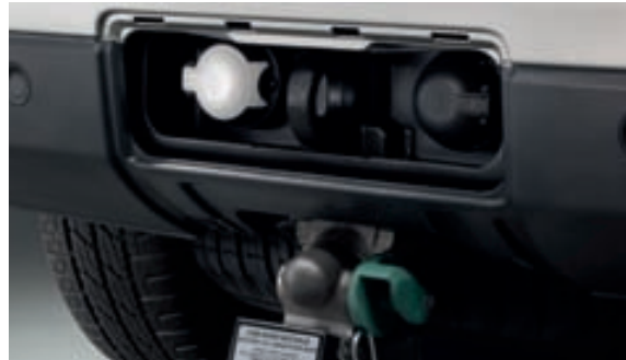
'N' and 'S' Type Towing Electrics** VPLAT0011 Provides all trailer rear lighting and interior equipment power, where required. Standard fit all models.
