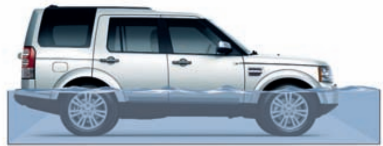
Wading Depth Maximum wading depth 700mm (air suspension only) Normal wading depth 600mm
