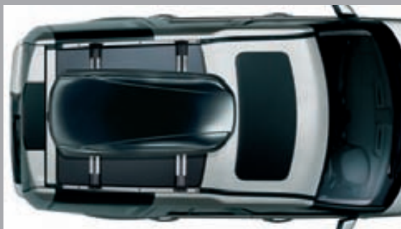
Luggage Box* VPLVR0062 Gloss Black Finish. Opens from both sides. Lockable for security. External dimensions: 1,750mm long, 820mm wide, 450mm high. Internal volume 440 litres. Load capacity 75kg † .
