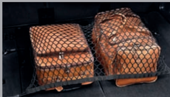
Load Retention Net VUB503130 Utilises loadspace tie-down points. Includes floor net and two ratchet straps. Strap length approximately 2 metres.
