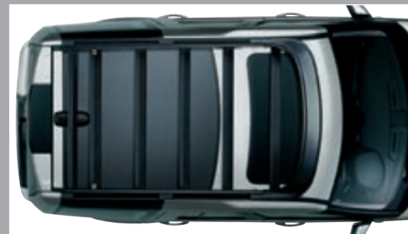
Expedition Roof Rack* CAB500021PMA Vehicle must be fitted with a Short Roof Rail Kit CAB500120PVJ (not shown)/CAP500090. Vehicle height when fitted 2,100mm at normal ride height, Load capacity 54.3kg † .
