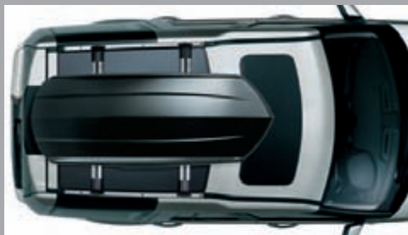
Sports Box* VPLVR0061 Gloss Black Finish. Can be mounted either side for kerbside opening in any country. Internal retention system for skis or other long loads. Lockable for security. External dimensions: 2,060mm long, 840mm wide, 340mm high. Internal volume 420 litres. Load capacity 75kg † .
