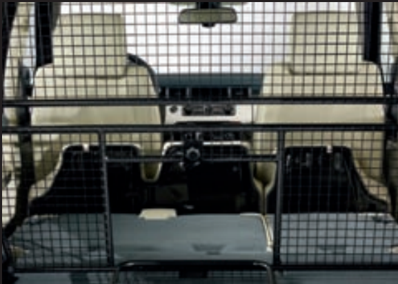
Dog Guard* VUB502080 Easily removed, incorporates useful integral ski hatch.
