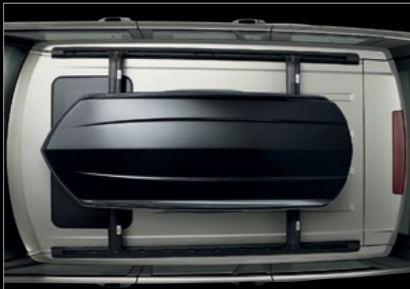
Sports Box* VPLVR0061 Gloss Black finish. Can be mounted on either side of the vehicle for kerbside opening in any country. Internal retention system for skis or other long loads. Lockable for security. External dimensions: 2,060mm long, 840mm wide, 340mm high. Volume 420 litres. Load capacity 75kg.
