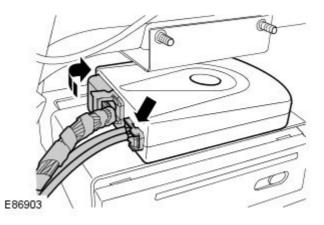
5. ONOTE: Electrical connection not required, remove for access only.
