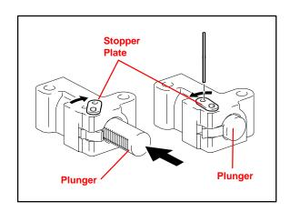
C. Install the No. 1 chain tensioner assembly with the 2 bolts.
