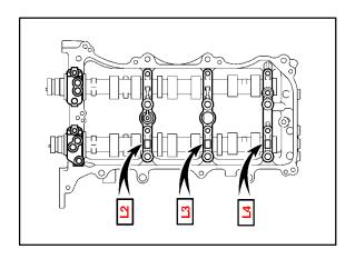
D. Tighten the 8 M6 bolts in the sequence shown in the illustration.
