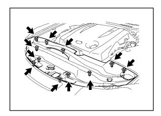
3. Remove the engine compartment side cover LH by removing the 5 clips.
