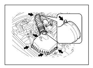
10. Remove the air cleaner case sub-assembly by removing the 2 bolts and clamp.
