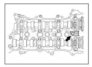
C. While holding the No. 2 chain, slide the No. 2 camshaft out toward the front of the vehicle.
