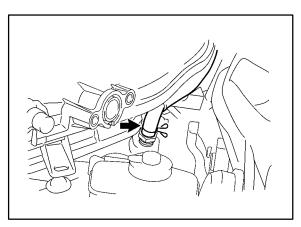
E. Remove the bolt and water hose joint from the intake air surge tank.
