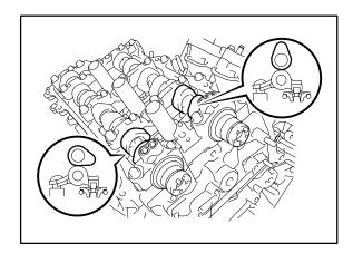
B. Uniformly loosen and remove the 9 camshaft bearing cap M6 bolts in the sequence shown in the illustration.
