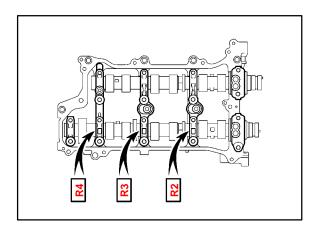
D. Tighten the 9 M6 bolts in the sequence shown in the illustration.
