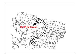
21. Remove No. 2 oil pipe union bolt from the oil pipe.
