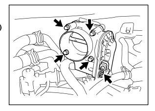
57. Connect the No. 2 fuel vapor hose. Install the clamp and connect the No. 2 fuel vapor feed hose.
