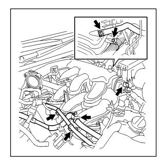
H. Connect the No. 1 vacuum switching valve assembly to the intake air surge tank.
