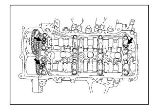
D. Install the head cover with the 12 bolts.
