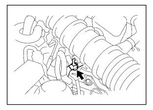
C. Connect the MAF connector and clamp to the air cleaner.
