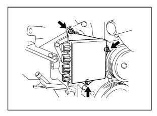
26. Remove the timing chain cover plate by removing the 4 bolts, timing chain cover plate, and timing chain cover plate gasket.
