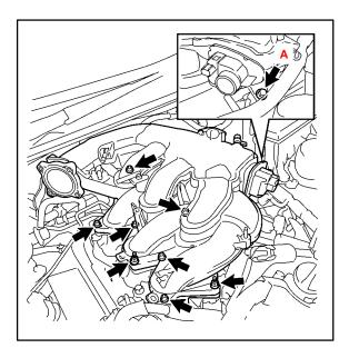
D. Install the surge tank stay to the intake air surge tank.
