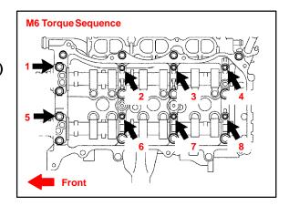
E. Tighten the 8 M8 bolts in the sequence shown in the illustration.
