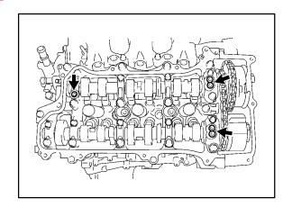
D. Install the head cover with the 14 bolts.
