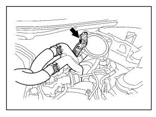
F. Connect the ventilation hose to the intake air surge tank.
