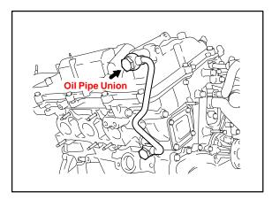
49. Install the oil pipe union bolt to the No. 1 oil pipe.
