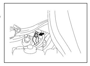
E. Connect the water hose joint with the bolt.
