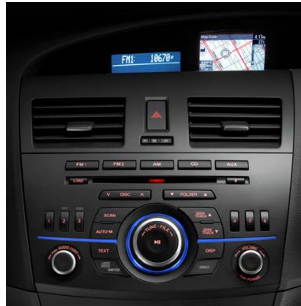
Control room. Multi information display shows everything from audio and fuel economy info to service reminders. Maxx Sport and up feature a colour 4.1 inch screen incorporating easy-to-use sat nav, plus an in-dash single disc MP3 compatible CD player.
