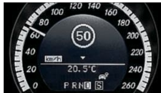
Speed Limit Assist even warns you about temporary speed limits
