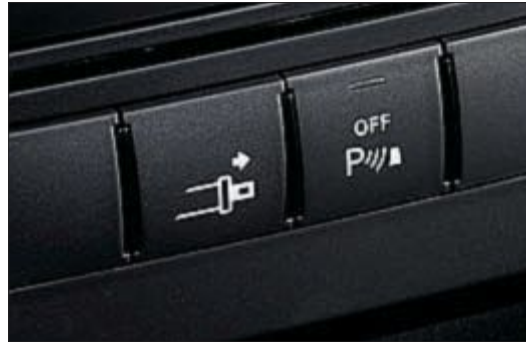
Button on centre console for belt feeder
