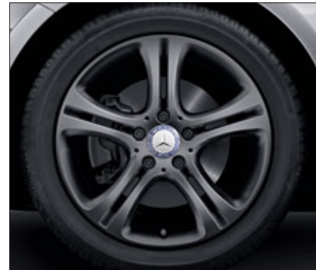
5-twin-spoke light-alloy wheels, painted tremolite grey, with 225/45 R 17 tyres (option, Code 44R).
