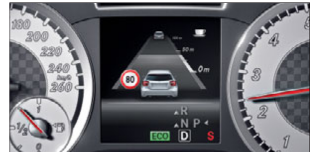
The information from Speed Limit Assist is shown both in the instrument cluster and in the COMAND Online central display.
