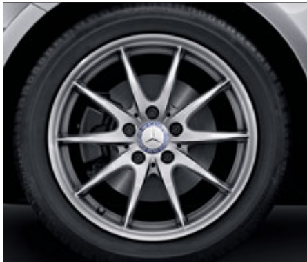
10-spoke light-alloy wheels with 225/45 R 17 tyres (standard for A 220 CDI, A 250 and A 250 4MATIC, Code R43).
