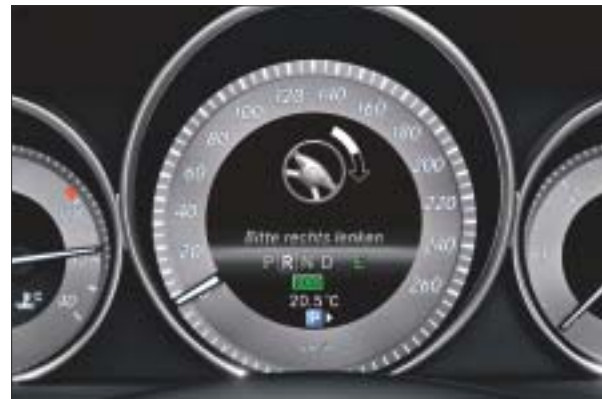
The display in the instrument cluster gives you a clear picture of what is happening at all times when parking
