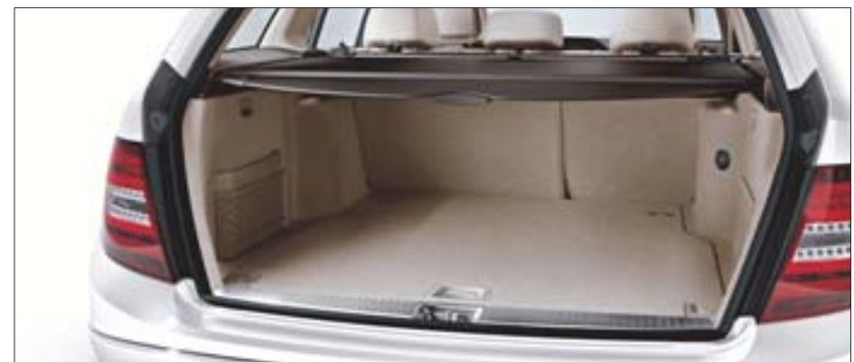
The load compartment cover shields the contents of the luggage compartment from the sun's rays and from prying eyes
