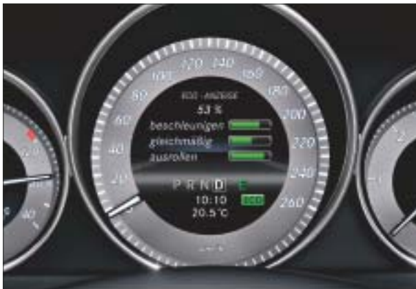
The ECO display provides feedback about the efficiency of the driving style
