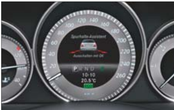
Active Lane Keeping Assist can make the steering wheel vibrate if the vehicle drifts unintentionally across lane markings
