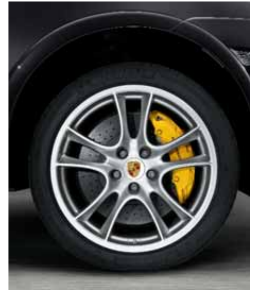
Porsche Ceramic Composite Brake (PCCB)
