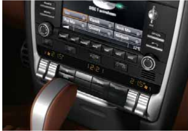
Air-conditioning controls (cover open)
