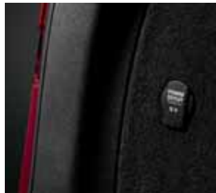
12-Volt power point in luggage compartment
