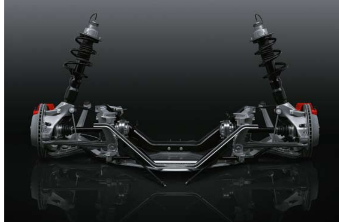
Lightweight spring-strut rear axle on the Cayman S
