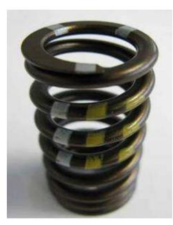
If this spring is fitted, replace the exhaust valve springs according to the repair manual.
