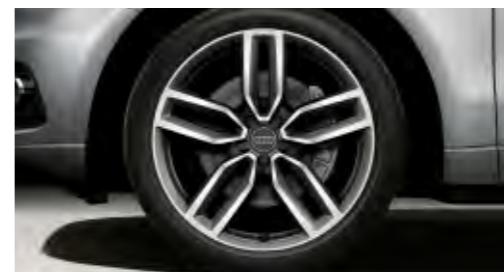
Audi exclusive cast aluminium wheels in 5-twin-spoke star design in titanium look, high-gloss turned finish size 8.5 J x 21 with 255/40 R 21 tyres, including wheel arch trims. From quattro GmbH
