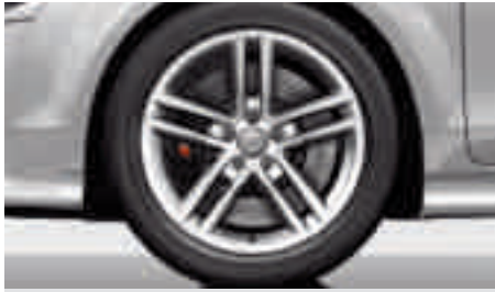
Cast aluminium wheels, 5-double-spoke design, size 9 J x 18 with 245/40 R 18 tyres
