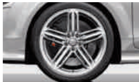
Cast aluminium wheels, 5-segment-spoke design, size 9 J x 19 with 255/35 R 19
