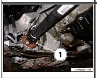
3. Rotate the driveshaft 90° and repeat steps 1 and 2. Rotate the driveshaft another 90° and recheck for play. Rotate a total of four times (the driveshaft has now been rotated 360° total).
