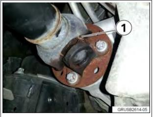
2. There should be no exposed needle bearings (1).
