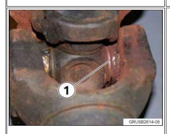
3. There should be no excessive rust at the bearing seals (1). Note: There will be rust buildup on the driveshaft and mounting flange on some driveshafts. This rust is normal. Only excessive rust on the bearing seals indicates the seal may fail.
