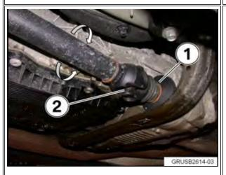
2. Checking the rear U-joint:
