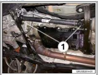
Check the universal joints in the front driveshaft for radial play (1).
