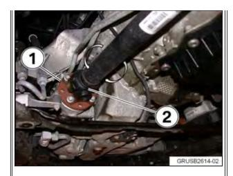
Hold the input flange (1) on the front differential and check for radial play in the U-joint (2).
