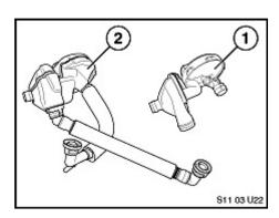
1. Replace the oil separator and hoses (1) with the new insulated style (2).
