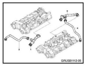
Each of the connecting lines will have an index number printed on the connection closest to the cylinder head cover.
