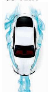
After an extensive programme of advanced computer simulations, the Supersports' engineering team calculated that an increase in turbocharger boost would require a 10 percent increase in airflow to the twin intercoolers and cooling system, thus allowing the engine to generate its extra power and torque.
