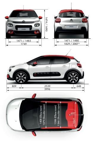
\* vehicle width/width with slide mirrors out.
