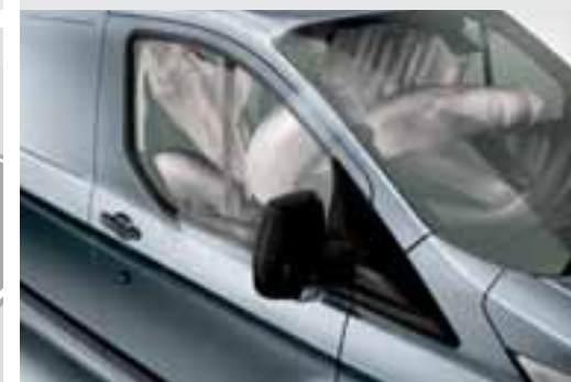
Six Airbags Standard All Transit Commercial Vehicles feature airbags positioned at the front, on both sides and at the head to enhance protection of the driver and front passengers in the event of an accident.
