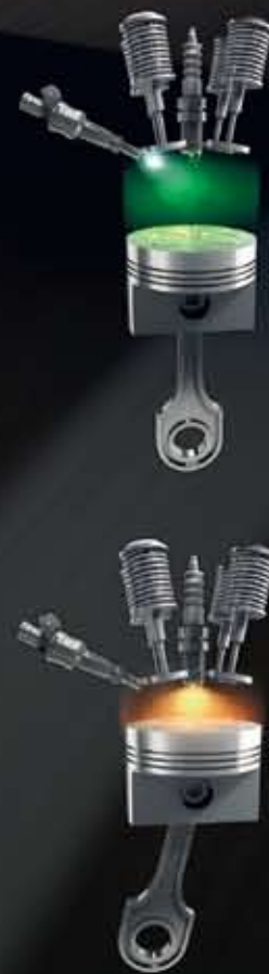
SIDI technology injects fuel directly into the cylinder, increasing power while saving fuel
