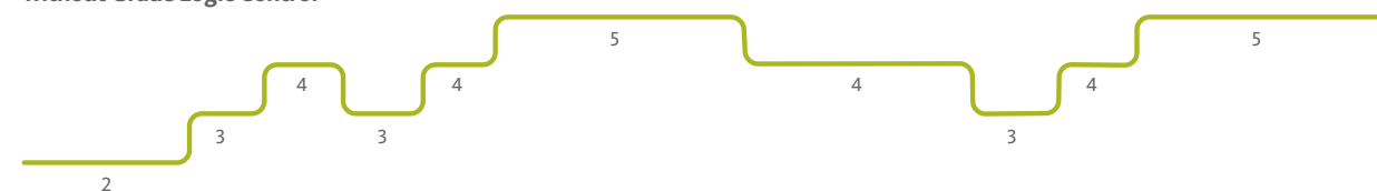
Typical 'gear hunting' without Grade Logic Control
