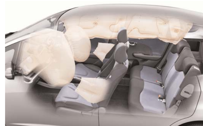
Picture shows deployed driver and passenger side SRS airbag system, front-seat i-side airbag system and side curtain airbag system.
