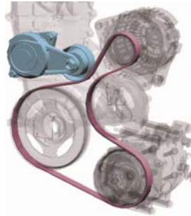
Auxiliary belt drive system configuration
