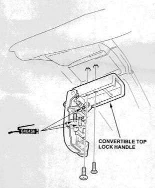
Install the handle(s) in the reverse order of removal, and apply multipurpose grease to its springs and moving parts. Then, go to step 11.  Locate the burrs at the right-rear of the frame hinge, then use a file to remove the burrs and any rough areas.
