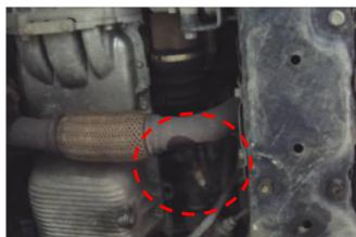
3. Remove the front muffler assembly by removing the front and rear mounting nuts.
