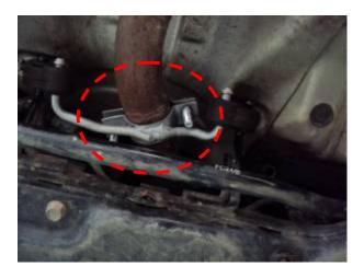
6. Check to verify that the bracket is tight and that the bracket does not slide along the exhaust pipe.
