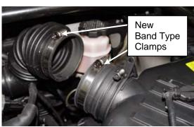
7. Reinstall the Mass Air Flow Sensor and tighten the new hose clamps.
