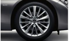
18 X 7.5-INCH, ALUMINUM-ALLOY WHEELS STANDARD ON Q50 PURE MODELS.
