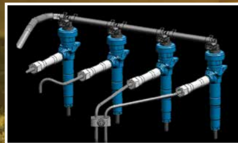
Improved redesign of fuel injector pintle caps for optimum fuel efficiency
