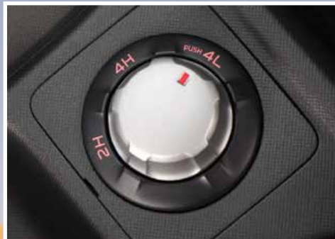
"Terrain Command" 4WD system allows for simple shift from 2WD high, 4WD high and 4WD low
