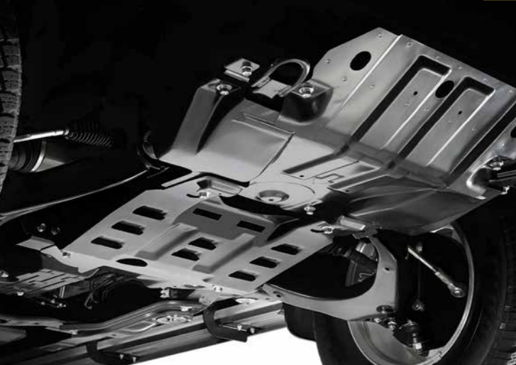
Underbody protection, front steel plate skid/shield
