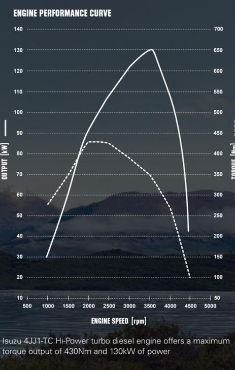
Isuzu 4JJ1-TC Hi-Power turbo diesel engine offers a maximum torque output of 430Nm and 130kW of power
