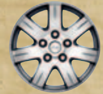
17-inch cast aluminium with machined face
