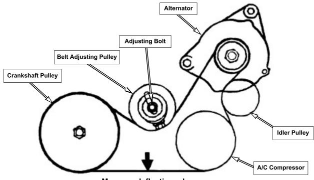
Measure deflection when applying 20-22 lbs of force in the direction of the solid black arrow in above illustration.
