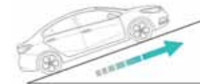
Hill-start Assist Control (HAC) By maintaining brake grip until you press the accelerator, HAC prevents the vehicle from dangerously rolling backwards when pulling away from a standstill on an incline.
