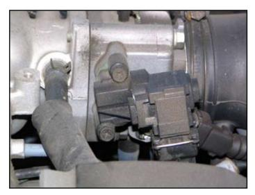
3. Disconnect the throttle position sensor (TPS) connector and remove the two (2) mounting screws.
