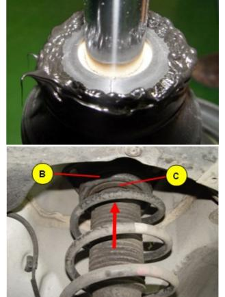
5. Push up the dust cover (B) to reach the insulator assembly (C).
