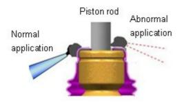
4-2. Turn the dust cover applying urethane sealant all round the dust cover.
