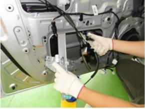
14. Remove the 3 power window motor mounting bolts, and then separate the power window motor from the regulator.
