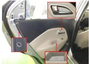
5. Remove the rear door inside handle housing (B).
