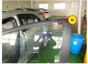
12. Disconnect the power window regulator motor connector (I), then remove the 6 window regulator mounting bolts (10 mm).
