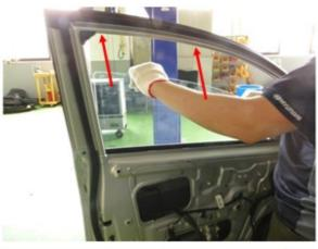
11. Fix the window glass with the tape (H) as shown in the image to prevent it from sliding down
