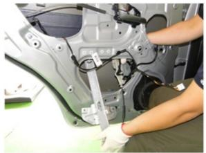
14. Install the new regulator assembly (K) in reverse order of the removal.
