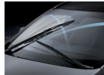
Opposed-type wiper system Unlike conventional wiper systems, the wiper blades are mounted on opposite sides of the windshield and move in the opposite direction for maximum visibility even in heavy rain and snow.
