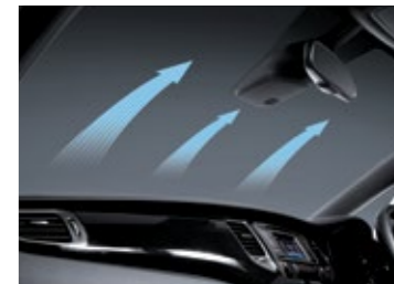
Auto defogging system A sensor automatically initiates a defogging process when condensation is detected on the windows to ensure optimal visibility in humid climates. (SLi & Platinum)
