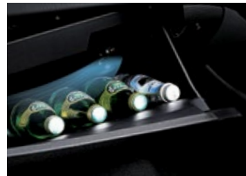
Cooled glove box The large 8L glove box has a cooling function that comes in handy when storing perishable items or cold drinks, especially on long journeys. (Platinum)
