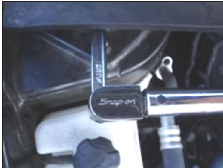
Front strut upper nut tightening procedure
