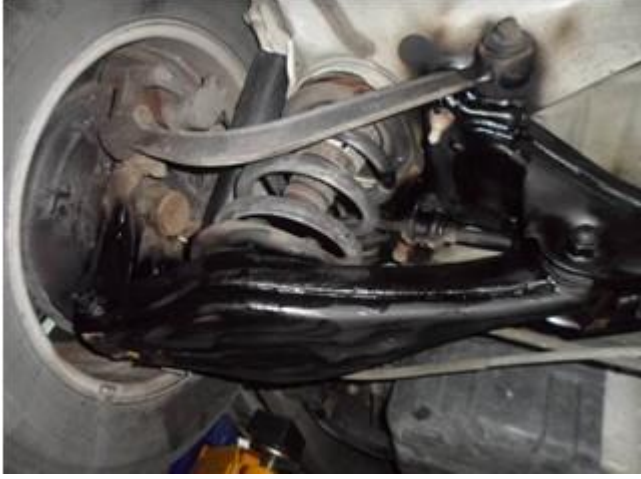
Finished View Spraying Under Coating To Rear Cross Member & Rear Lower Arm
