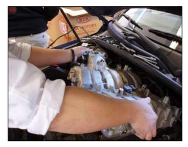
14. Using a clean work surface, remove the Intake Control Valve (ICV) from the Surge Tank.
