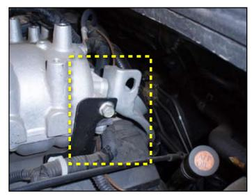
11. Remove the front stay bracket from the intake manifold assembly.
