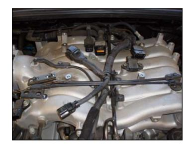
4. Remove and re-position the steel coolant transfer line.
