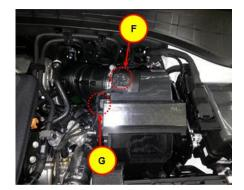
5. Remove the hydraulic electronic control unit connector.
