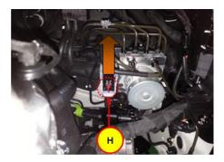
6. Check again if the ground bolt / cable (I) is installed to the body panel.
